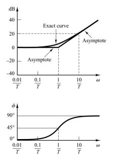
**Figure 7–8** Log-magnitude curve, together with the asymptotes, and phase-angle curve for  $1 + j\omega T$ .
