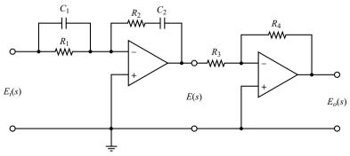
**Figure 8–70** Electronic PID controller.
