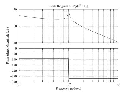
Figure 8–14 Bode diagram of  $4/[s(s^2 + 1)]$ .
