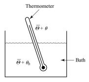
Figure 4-40 Thin, glass-wall, mercury thermometer system.
