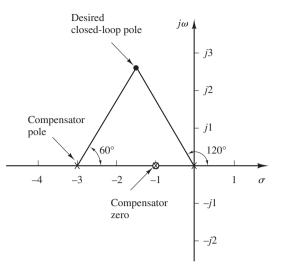
**Figure 6–44** Compensator pole and zero.
