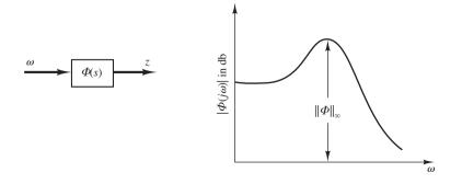
**Figure 10–41** Bode diagram and the  $H_{\infty}$  norm  $\|\Phi\|_{\infty}$ .
