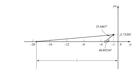
**Figure 6–80** Determination of the pole of the lead network.
