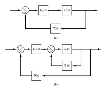
Figure 6–33 (a) Series compensation; (b) parallel or feedback compensation.
