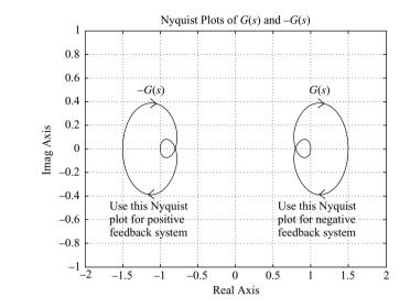
Figure 7–131 Nyquist plots for positive-feedback system and negativefeedback system.
