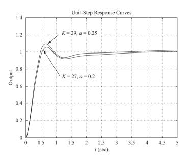
**Figure 8–65** Unit-step response curves.
