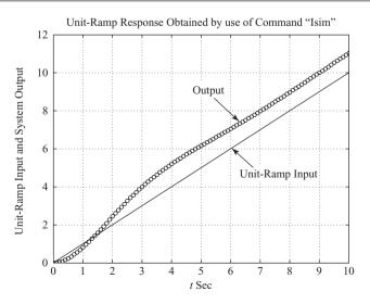
**Figure 5–28** Unit-ramp response.
