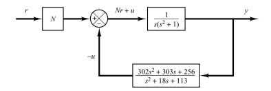
**Figure 10–31** Control system with observer controller in the feedback path.
