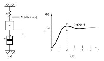
**Figure 5–54** (a) Mechanical vibratory system; (b) step-response curve.
