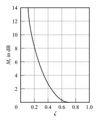
Figure 7–10  $M_r$ -versus- $\zeta$  curve for the second-order system  $1/[1 + 2\zeta(j\omega/\omega_n) + (j\omega/\omega_n)^2].$
