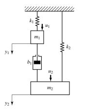
Figure 3–32 Mechanical system.
