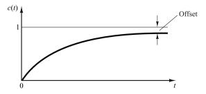
**Figure 5–38** Unit-step response and offset.
