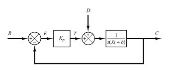
**Figure 5–40** Control system with a torque disturbance.
