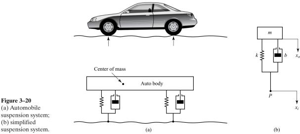
(b) simplified suspension system. **A-3-2.** Obtain the transfer function Y(s)/U(s) of the system shown in Figure 3–21. The input *u* is a displacement input. (Like the system of Problem **A-3-1**, this is also a simplified version of an automobile or motorcycle suspension system.)
