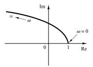
Figure 7-30 Polar plot of  $1 + 2\zeta \left(j \frac{\omega}{\omega_n}\right) + \left(j \frac{\omega}{\omega_n}\right)^2$  for  $\zeta > 0$ .
