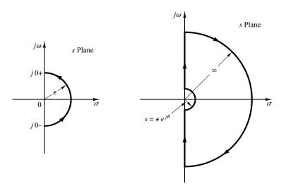
**Figure 7–50** Contour near the origin of the *s* plane and closed contour in the *s* plane avoiding poles and zeros at the origin.
