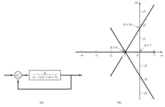
**Figure 6–69** (a) Control system; (b) root-locus plot.
