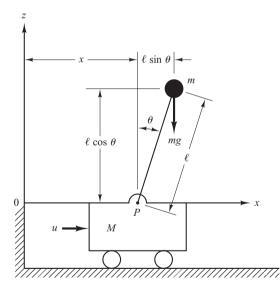
**Figure 10–59** Inverted-pendulum system.
