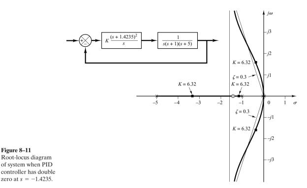
Figure 8–11 Root-locus diagram of system when PID controller has double
