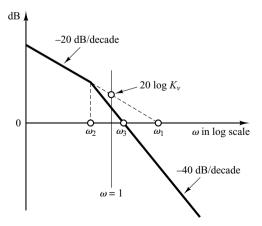
**Figure 7–18** Log-magnitude curve of a type 1 system.
