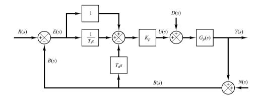
**Figure 8–26** PI-D-controlled system.
