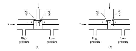
Figure 4–32 (a) Overlapped spool valve; (b) underlapped spool valve.
