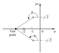
**Figure 6–8** Determination of the root locus on the real axis.
