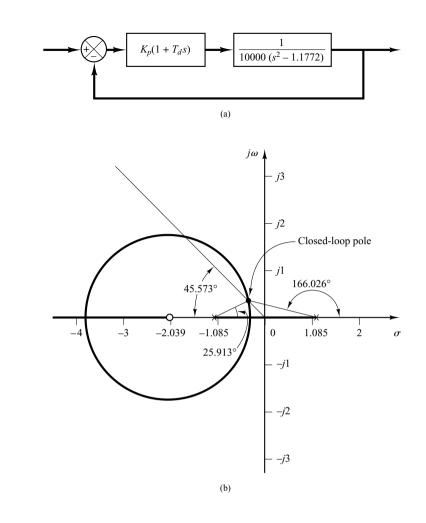
Figure 6–83 (a) PD control of an unstable plant; (b) root-locus diagram for the system.
