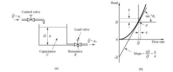
**Figure 4–1** (a) Liquid-level system; (b) head-versus-flow-rate curve.
