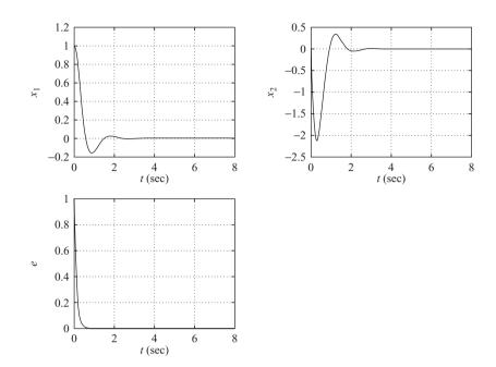
**Figure 10–53** Response curves to initial condition.
