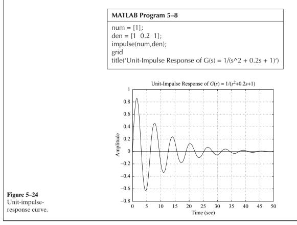
Alternative Approach to Obtain Impulse Response. Note that when the initial conditions are zero, the unit-impulse response of G(s) is the same as the unit-step response of sG(s).
