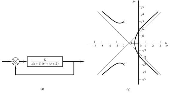
**Figure 6–68** (a) Control system; (b) root-locus plot.
