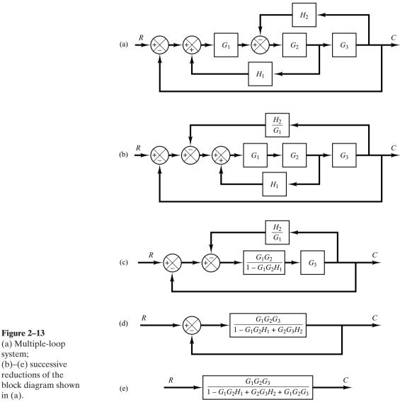
(b)-(e) successive reductions of the block diagram shown in (a).
