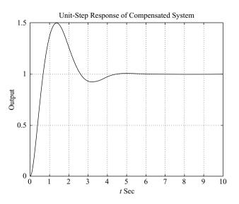
Figure 6–79 Unit-step response of the compensated system.
