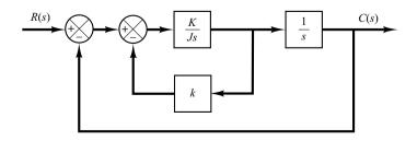
Figure 5–53 Closed-loop system.
