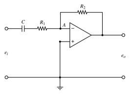
Figure 3–39 Operational-amplifier circuit.
