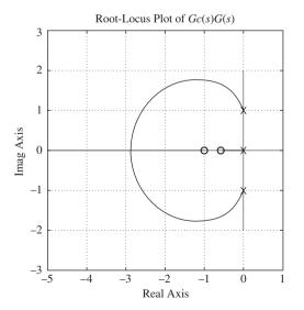
Figure 8–50 Root-locus plot of the compensated system.
