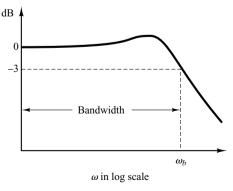
Figure 7–76 Plot of a closed-loop frequency response curve showing cutoff frequency  $\omega_b$  and bandwidth. The specification of the bandwidth may be determined by the following factors:
