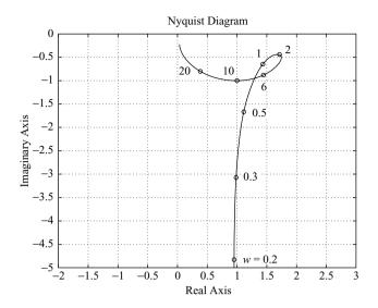
Figure 7–129 Polar plot of  $G(j\omega)$ given in Problem A–7–13.
