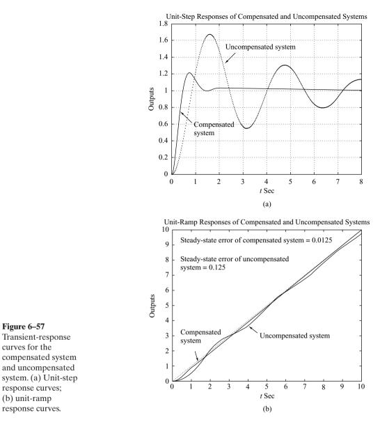
The unit-step response curves and unit-ramp response curves before and after compensation are shown in Figure 6–57. (Notice a long tail of a small amplitude in the unit-step response of the compensated system.)
