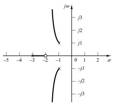
Figure 6–32 Root-locus plot for the negative-feedback system with  $G(s) = K(s + 2)/[(s + 3)(s^2 + 2s + 2)],$ H(s) = 1.
