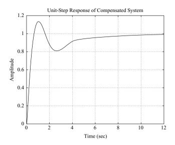
Figure 8–51 Unit-step response of the compensated system.
