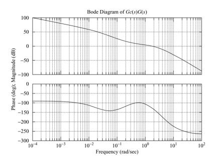
**Figure 7–153** Bode diagram of the open-loop transfer function  $G_c(s)G(s)$  of the compensated system.
