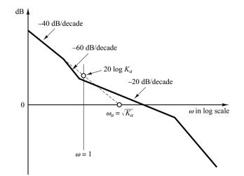
**Figure 7–19** Log-magnitude curve of a type 2 system.
