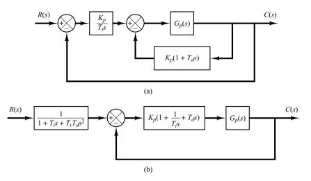
Figure 8–60 (a) I-PD-controlled system; (b) PID-controlled system with input filter.
