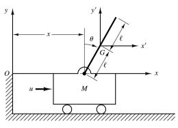
Figure 3–34 Inverted-pendulum system.
