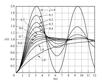
**Figure 5–7** Unit-step response curves of the system shown in Figure 5–6.
