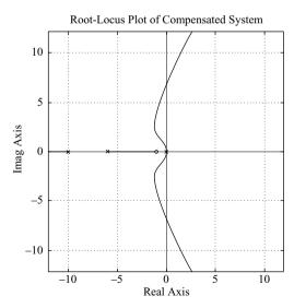
Figure 6–78 Root-locus plot of the compensated system.
