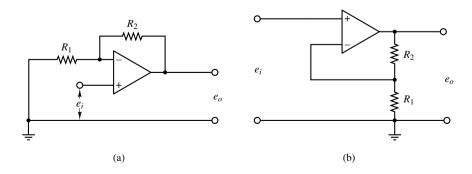
Figure 3–15 (a) Noninverting operational amplifier; (b) equivalent circuit.
