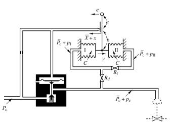
**Figure 4–30** Schematic diagram of a pneumatic controller. From the equations just derived, a block diagram of the controller can be drawn, as shown in Figure 4–31(a). Simplification of this block diagram results in Figure 4–31(b).
