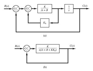
Figure 5–13 (a) Block diagram of a servo system; (b) simplified block diagram.
