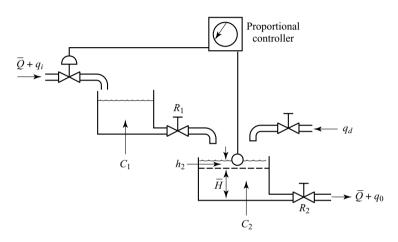
**Figure 4–43** Liquid-level control system.
