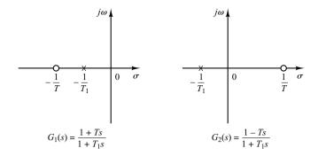
The pole–zero configurations of these systems are shown in Figure 7–12. The two sinusoidal transfer functions have the same magnitude characteristics, but they have different phase-angle characteristics, as shown in Figure 7–13. These two systems differ from each other by the factor
