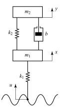
**Figure 3–21** Suspension system.
