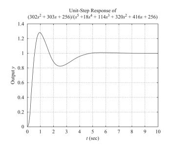
**Figure 10–30** Unit-step response of the control system shown in Figure 10–29.
