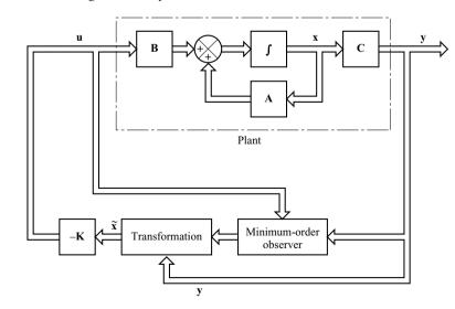
**Figure 10–16** Observed-state feedback control system with a minimum-order observer.
