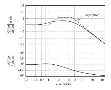
**Figure 7–118** Bode diagram for  $10(1 + j\omega)/[(2 + j\omega)(5 + j\omega)].$
