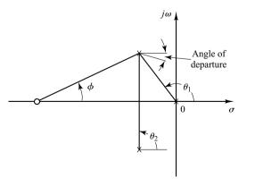
Figure 6–12 Construction of the root locus. [Angle of departure =  $180^{\circ} - (\theta_1 + \theta_2) + \phi$ .] of the root loci in this important region in the *s* plane must be obtained with reasonable accuracy. (If accurate shape of the root loci is needed, MATLAB may be used rather than hand calculations of the exact shape of the root loci.)
