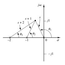
**Figure 6–5** Construction of root locus.
