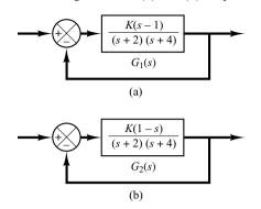
Figure 6-102 (a) and (b) Nonminimum-phase systems.
