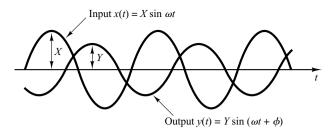
**Figure 7–2** Input and output sinusoidal signals.
