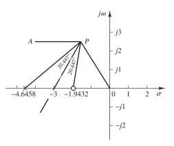
**Figure 6–42** Determination of the pole and zero of the lead compensator.
