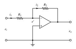
**Figure 3–14** Inverting amplifier.
