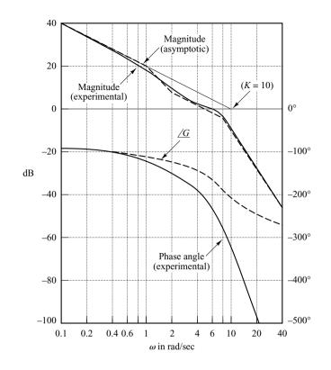
Figure 7–88 Bode diagram of a system. (Solid curves are experimentally obtained curves.)
