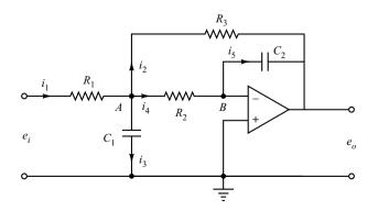
**Figure 3–28** Operationalamplifier circuit.
