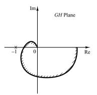
**Figure 7–49** Region enclosed by a Nyquist plot. Special Case when G(s)H(s) Involves Poles and/or Zeros on the  $j\omega$  Axis. In the previous discussion, we assumed that the open-loop transfer function G(s)H(s) has neither poles nor zeros at the origin. We now consider the case where G(s)H(s) involves poles and/or zeros on the  $j\omega$  axis.
