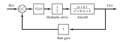
**Figure 6–94** Compensated attitude-rate control system.
