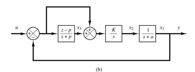
Figure 2–28 (a) Control system; (b) block diagram defining state variables for the system.
