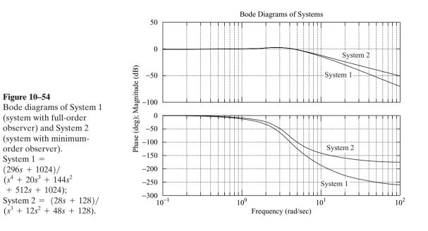
The observer controller is clearly a lead compensator.
