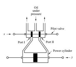
**Figure 4–19** Hydraulic servomotor.  $A\rho \, \frac{dy}{dt} = K_1 x$
