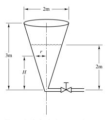
Figure 4-42 Conical water-tank system.
