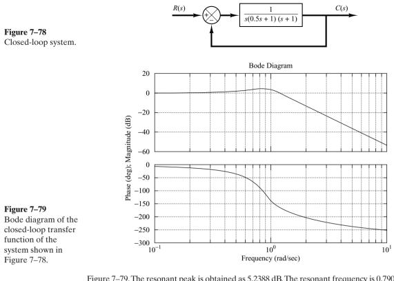
Figure 7–79. The resonant peak is obtained as 5.2388 dB. The resonant frequency is 0.7906 rad/sec. The bandwidth is 1.2649 rad/sec. These values can be verified from Figure 7–78.
