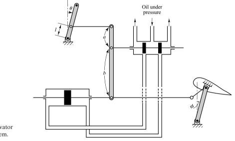
**Figure 4–51** Aircraft elevator control system.
