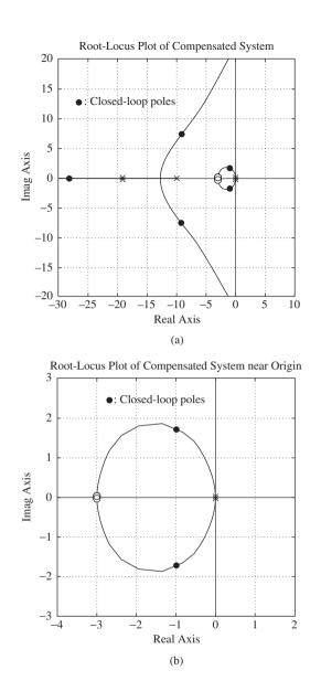
**Figure 6–81** (a) Root-locus plot of compensated system; (b) root-locus plot near the origin.
