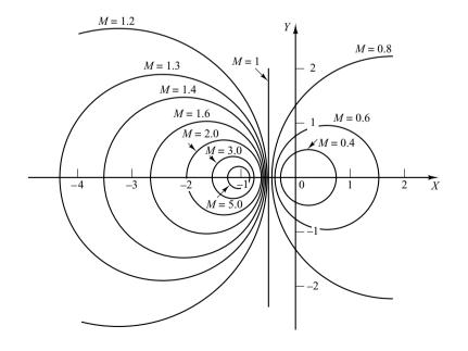
**Figure 7–81** A family of constant *M* circles. **Constant-Phase-Angle Loci** (*N* Circles). We shall obtain the phase angle  $\alpha$  in terms of X and Y. Since
