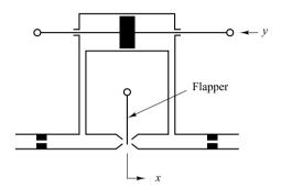
diagram of the system of Figure 4–50 and then find the transfer function between y and x, where x is the air pressure and y is the displacement of the power piston.
