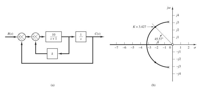
Figure 6–99 (a) Control system; (b) root-locus plot, where K = 10k. Notice that the system has a zero at s = 0 and two poles at  $s = -0.5 \pm j3.1225$ . Since this system involves two poles and one zero, there is a possibility that a circular root locus exists. In fact, this system has a circular root locus, as will be shown. Since the angle condition is
