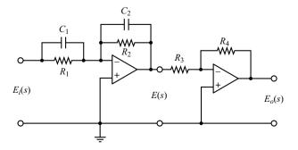
Figure 6–36 Electronic circuit that is a lead network if  $R_1C_1 > R_2C_2$  and a lag network if  $R_1C_1 < R_2C_2$ .
