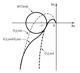
Figure 7–90 Reshaping of the open-loop frequency-response curve.
