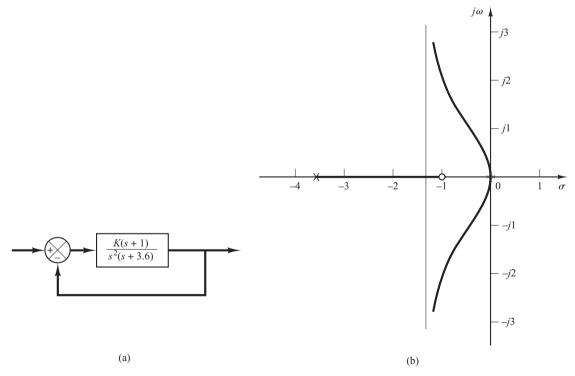
Figure 6–65 (a) Control system; (b) root-locus plot.
