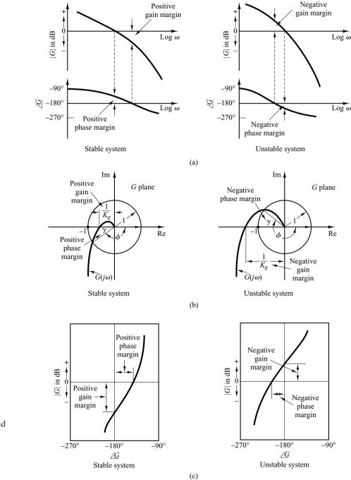
Figure 7–67 Phase and gain margins of stable and unstable systems. (a) Bode diagrams; (b) polar plots; (c) log-magnitudeversus-phase plots.
