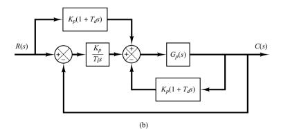
**Figure 8–72** (a) PID-controlled system; (b) I-PD-controlled system with feedforward control.
