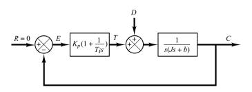
Proportional-plusintegral control of a load element consisting of moment of inertia and viscous friction.
