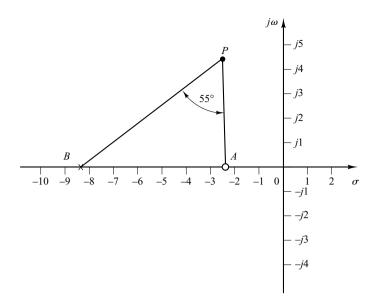
**Figure 6–58** Determination of the desired pole-zero location.
