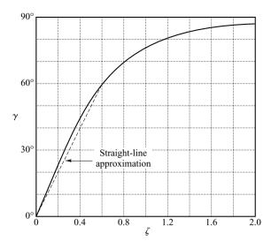
**Figure 7–74** Curve  $\gamma$  (phase margin) versus  $\zeta$  for the system shown in Figure 7–73.
