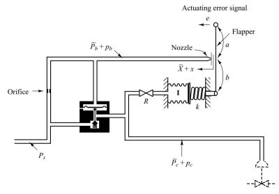
**Figure 4–46** Pneumatic controller.
