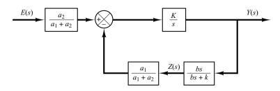
Figure 4–36 Block diagram for the speed control system shown in Figure 4–35.
