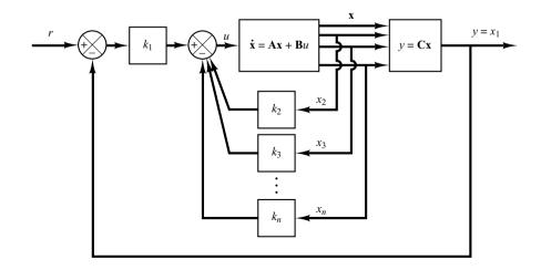
**Figure 10–4** Type 1 servo system when the plant has an integrator. the reference input *r* is a step function. In this system we use the following state-feedback control scheme:
