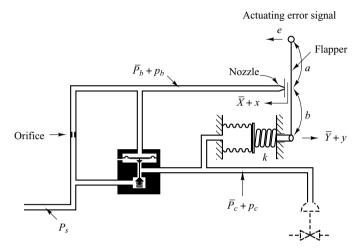
**Figure 4–45** Pneumatic controller.
