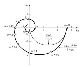
**Figure 7–126** Polar plots of  $2.65e^{-0.8j\omega}/(1 + j\omega)$  and  $2.65/(1 + j\omega)$ . A-7-11. Consider a unity-feedback system with the following open-loop transfer function:
