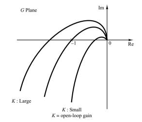
Figure 7-66 Polar plots of  $\frac{K(1 + j\omega T_a)(1 + j\omega T_b)\cdots}{(j\omega)(1 + j\omega T_1)(1 + j\omega T_2)\cdots}.$  Figures 7–67(a), (b), and (c) illustrate the phase margin of both a stable system and an unstable system in Bode diagrams, polar plots, and log-magnitude-versus-phase plots. In the polar plot, a line may be drawn from the origin to the point at which the unit circle crosses the  $G(j\omega)$  locus. If this line lies below (above) the negative real axis, then the
