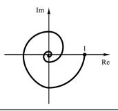
**Figure 7–32** Polar plot of  $e^{-j\omega L}/(1 + j\omega T)$ . General Shapes of Polar Plots. The polar plots of a transfer function of the form
