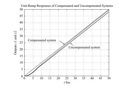
**Figure 6–51** Unit-ramp responses of compensated and uncompensated systems. [The compensator is given by Equation (6–20).]
