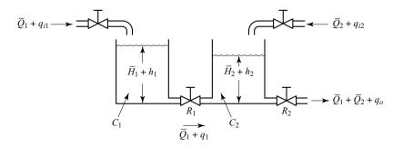
**Figure 4–28** Liquid-level system.
