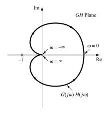
**Figure 7–53** Polar plot of  $G(j\omega)H(j\omega)$  considered in Example 7–14.
