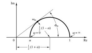
**Figure 7–91** Polar plot of a lead compensator  $\alpha(j\omega T + 1)/(j\omega\alpha T + 1)$ , where  $0 < \alpha < 1$ .
