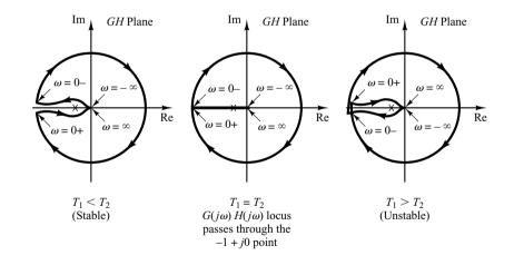
**Figure 7–55** Polar plots of the system considered in Example 7–16.
