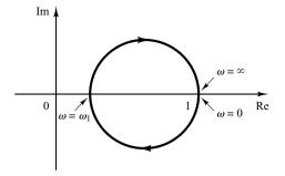
Polar plot of a lag-lead compensator given by Equation (7–27), with  $K_c = 1$  and  $\gamma = \beta$ .
