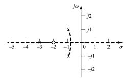
one real root enters the right-half *s* plane. Hence, for values of *K* greater than 3, the system becomes unstable. (For K > 3, the system must be stabilized with an outer loop.)
