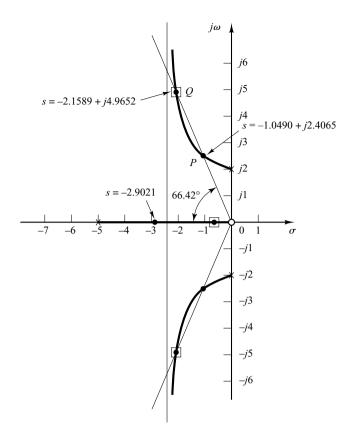
**Figure 6–62** Root-locus plot for the system shown in Figure 6–61.
