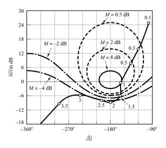
**Figure 7–142** Log-magnitudeversus-phase plot of G(s) given by Equation (7–32).
