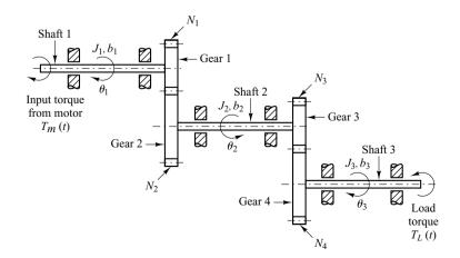
**Figure 5–51** Gear-train system.
