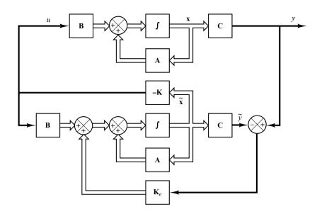
Figure 10–12 Observed-state feedback control system.
