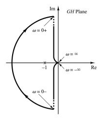
**Figure 7–56** Polar plot of the system considered in Example 7–17.
