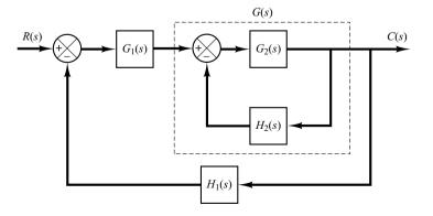
**Figure 7–59** Multiple-loop system.
