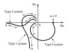
**Figure 7–33** Polar plots of type 0, type 1, and type 2 systems.
