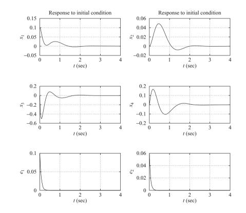
**Figure 10–50** Response curves to initial condition.
