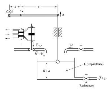
**Figure 4–52** Liquid-level control system.
