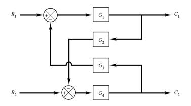
**Figure 2–24** System with two inputs and two outputs. Solution. From the figure, we obtain
