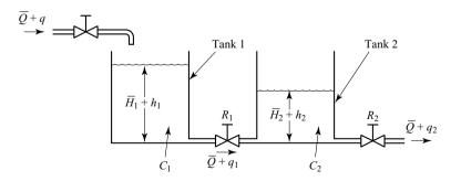
**Figure 4–2** Liquid-level system with interaction.
