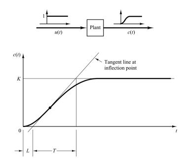
**Figure 8–2** Unit-step response of a plant.
