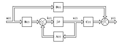
the operating state are discussed in Section 2–7.) A block diagram representation of Equations (2-12) and (2-13) is shown in Figure 2–14.
