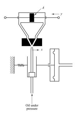
**Figure 4–34** Hydraulic jet-pipe controller.
