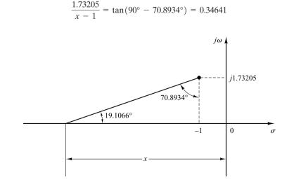
**Figure 6–77** Determination of the pole of the lead network.
