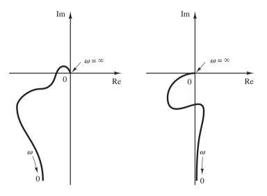
Figure 7–35 Polar plots of transfer functions with numerator dynamics.
