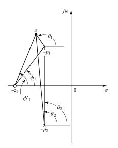
**Figure 6–9** Determination of the angle of departure.
