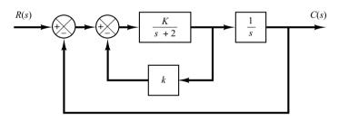
Figure 5–75 Closed-loop system.
