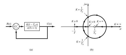
**Figure 6–26** (a) Nonminimumphase system; (b) root-locus plot.
