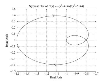
**Figure 7–130** Nyquist plot for positive-feedback system.
