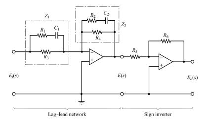
**Figure 6–53** Lag–lead compensator.
