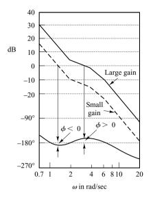
**Figure 7–108** Bode diagram of a conditionally stable system.
