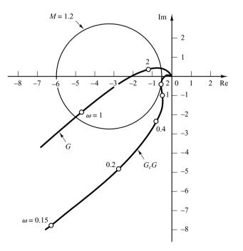
**Figure 7–112** Polar plots of G (gain adjusted) and  $G_cG$ .
