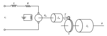
Figure 3-42 Armature-controlled dc servomotor system.
