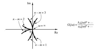
**Figure 7–34** Polar plots in the high-frequency range.
