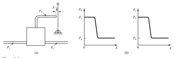
Figure 4–9 (a) Pneumatic controller without a feedback mechanism; (b) curves  $P_b$  versus X and  $P_c$  versus X.
