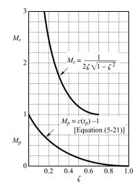
**Figure 7–75** Curves  $M_r$  versus  $\zeta$  and  $M_p$  versus  $\zeta$  for the system shown in Figure 7–73.
