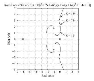
Figure 6–25 Root-locus plot of conditionally stable system.
