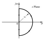
**Figure 7–47** Closed contour in the *s* plane.
