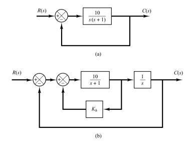
Figure 5–74 (a) Control system; (b) control system with tachometer feedback.
