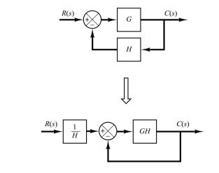
**Figure 7–62** Modification of a system with feedback elements to a unityfeedback system.
