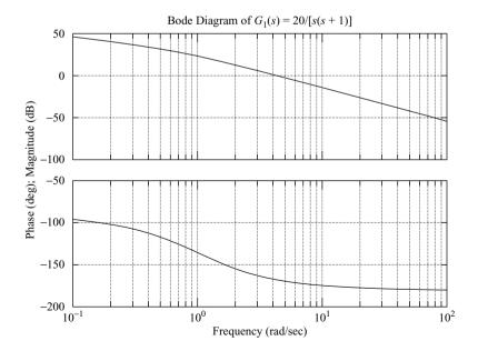
**Figure 7–145** Bode diagram of  $G_1(s)$ .
