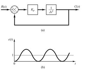
Figure 5–43 (a) Proportional control of a system with inertia load; (b) response to a unit-step input.
