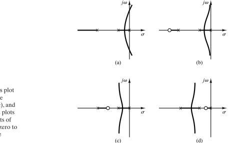
Figure 6–35 (a) Root-locus plot of a three-pole system; (b), (c), and (d) root-locus plots showing effects of addition of a zero to the three-pole
