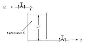
Figure 4–27 Liquid-level system.
