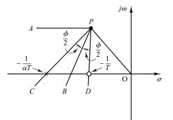
**Figure 6–41** Determination of the pole and zero of a lead network. Thus, if we need to force the root locus to go through the desired closed-loop pole, the lead compensator must contribute  $\phi = 40.894^{\circ}$  at this point. By following the foregoing design procedure, we can determine the zero and pole of the lead compensator.
