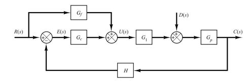
**Figure 2–23** Control system with reference input and disturbance input. By substituting Equation (2-47) into Equation (2-48), we get
