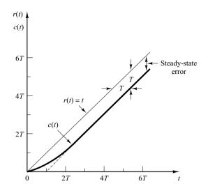
**Figure 5–3** Unit-ramp response of the system shown in Figure 5–1(a).
