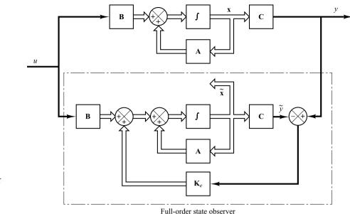
**Figure 10–11** Block diagram of system and full-order state observer, when input *u* and output *y* are scalars.
