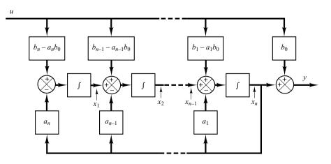
**Figure 9–2** Block diagram representation of the system defined by Equations (9–78) and (9–79) (observable canonical form). **A–9–3.** Consider the transfer-function system defined by
