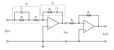
**Figure 8–45** Modified PID controller.
