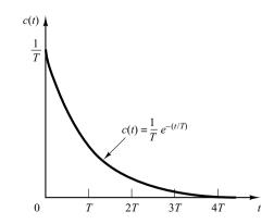
**Figure 5–4** Unit-impulse response of the system shown in Figure 5–1(a). An Important Property of Linear Time-Invariant Systems. In the analysis above, it has been shown that for the unit-ramp input the output c(t) is
