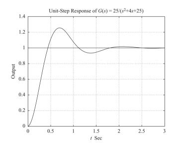
**Figure 5–21** Unit-step response curve.
