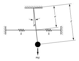
Figure 3–33 Spring-loaded pendulum system.
