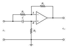
Figure 3–41 Operational-amplifier circuit.
