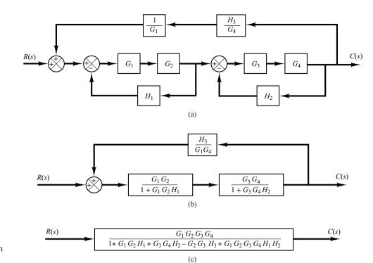
**Figure 2–22** Successive reductions of the block diagram shown in Figure 2–21.
