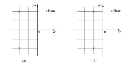
**Figure 7–64** Two systems with two closed-loop poles each.
