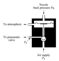
**Figure 4–7** Reverse-acting relay.
