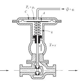
**Figure 4–11** Schematic diagram of a pneumatic actuating valve. where  $X(s) = \mathcal{L}[x]$  and  $P_c(s) = \mathcal{L}[p_c]$ . If  $q_i$ , the change in flow through the pneumatic actuating valve, is proportional to x, the change in the valve-stem displacement, then
