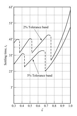
**Figure 5–11** Settling time  $t_s$  versus  $\zeta$  curves.
