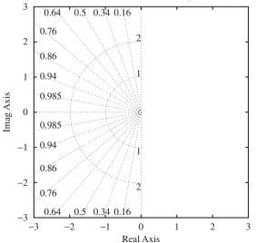
**Figure 6–22** Constant  $\zeta$  lines and constant  $\omega_n$  circles.
