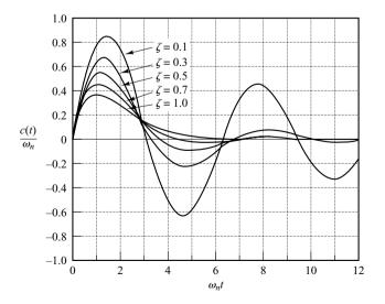
**Figure 5–14** Unit-impulse response curves of the system shown in Figure 5–6.
