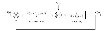
Figure 8–47 PID-controlled system. Design a control system such that the response to any step disturbance will be damped out quickly (in 2 to 3 sec in terms of the 2% settling time). Choose the configuration of the closed-loop poles such that there is a pair of dominant closed-loop poles. Then obtain the response to the unit-step disturbance input. Also, obtain the response to the unit-step reference input.
