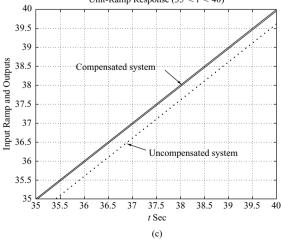
Figure 6–85 (a) Unit-step responses of the compensated and uncompensated systems; (b) unitramp responses of both systems; (c) unit-ramp responses showing steady-state errors.
