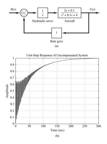
Figure 6–93 (a) Attitude-rate control system; (b) unit-step response.
