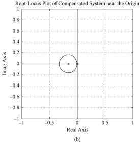
Figure 6–91 (a) Root-locus plot of compensated system; (b) rootlocus plot near the origin.
